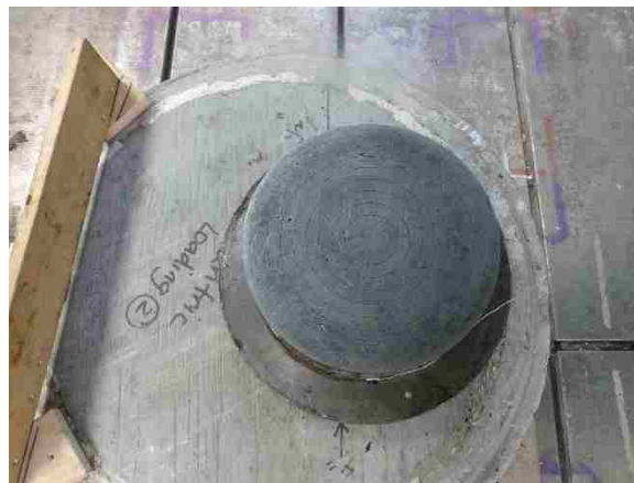
Figure 4-7. Load Bearing Plate shifted off-center for Eccentric Load Test
