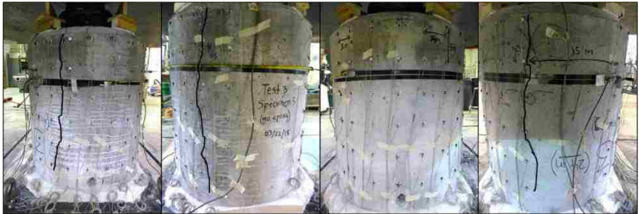
Figure 5-9. Crack formation at peak load for Test ep0-2 (L-R: N-W-S-E)
