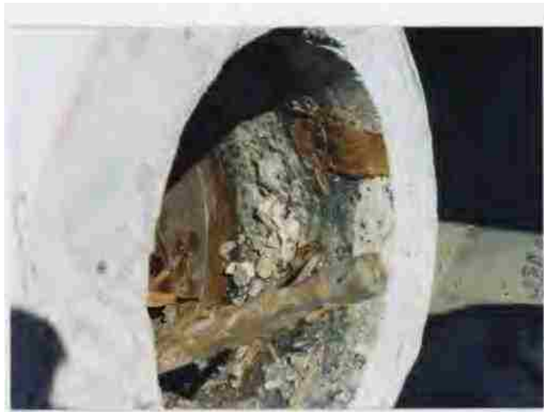
Figure 2-1. Internal spalling at core face of hollow specimen (Fig. 6.1.2., Budek, Benzoni and Priestley, 1997)
