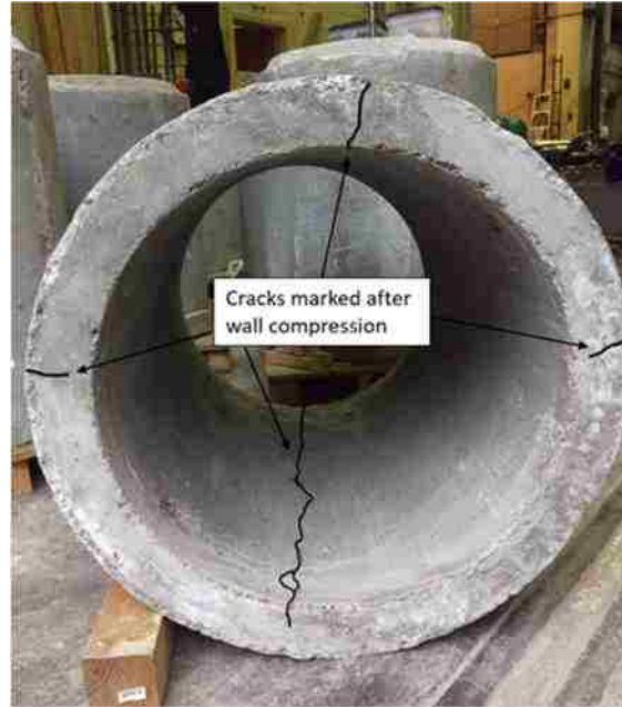
Figure 4-9. Longitudinal cracks - Specimen ep24-cr
