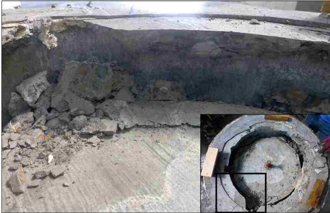
Figure 5-20. Plan View of Test ep24s4-1 at the end of testing showing "punching" displacement of plug
