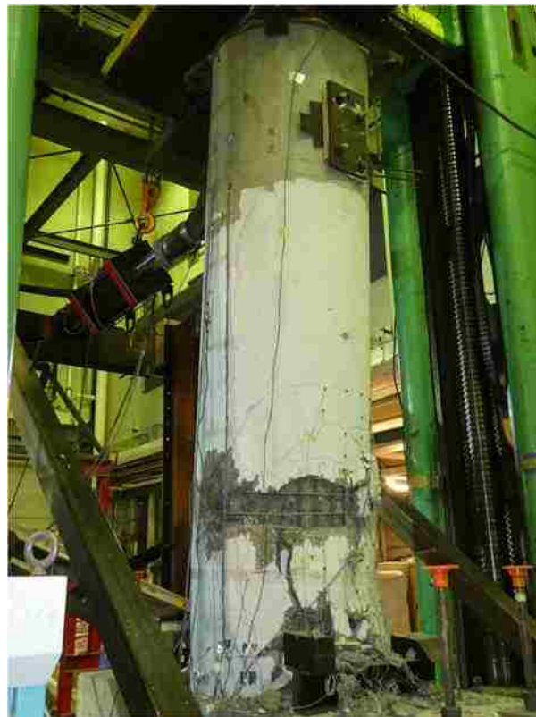
Figure 8-16. Final position of specimen at failure
