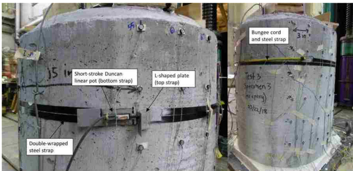
Figure 4-13. Instrumentation design to measure circumferential displacement
