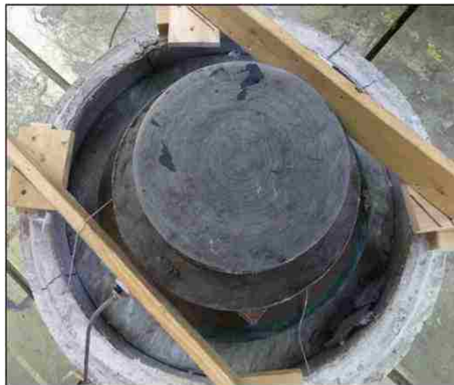
Figure 5-10. Plan view of Test ep0-2 at end of test showing no "punching" displacement (Similar for tests ep0-1 and ep24-2)
