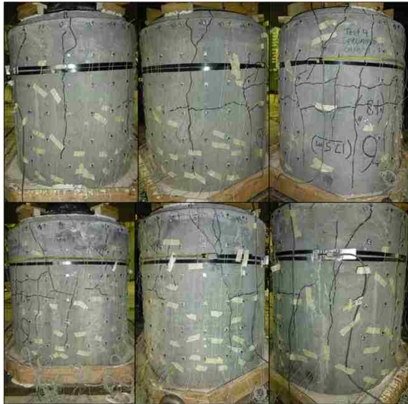
Figure 5-11. Crack formation at end of testing for Test ep18-1 (L-R: N-NW-SW; S-SE-NE)
