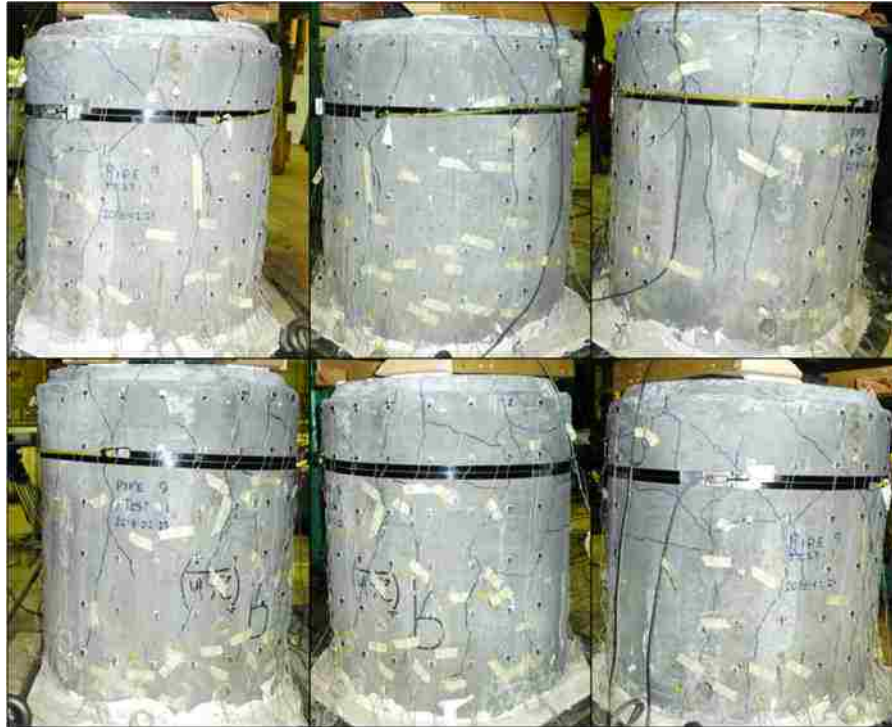
Figure 5-5. Crack formation at peak load for Test ep24-1 (L-R: N-NW-SW; S-SE-NE)
