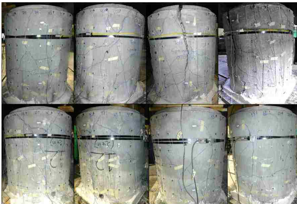
Figure 5-15. Crack formation at Peak Load for Test 9-ep24-ecc showing large crack on west side (L-R: N-NW-W-SW; S-SE-E-NE)
